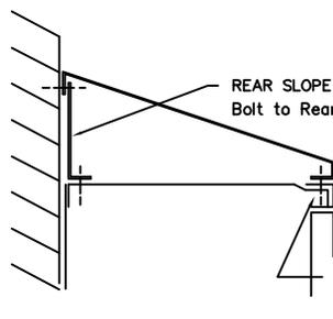
DETAIL OF SLOPE HOOD AT WALL
